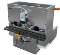
BRUSHING THE CABLE SHIELD
